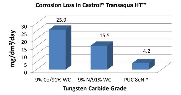
No company is more experienced than Penn United Technologies in supplying tungsten carbide oscillating and sliding valve seal faces for Oil and Gas subsea and subsurface controls. And Penn United's PUC-8eN<sup>™</sup> provides solutions to the challenges posed by today's aqueous control fluids while still providing the right mechanical properties for the most demanding control valve seal face requirements
