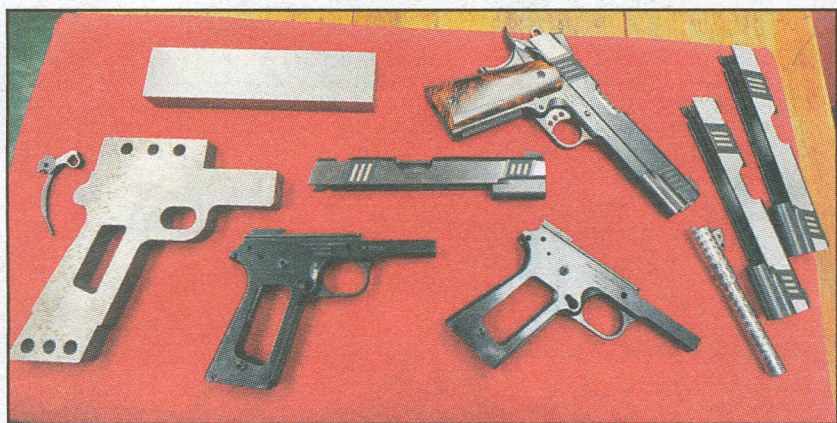
Parts at different stages of production for the Cabot Gun Co.'s 1911 models.
